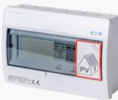
A complete certified switchboard protecting the DC line by max. voltage 1000 V. This type is intended for surface mounting and includes a two-pole fuse disconnector and a surge arrester to protect one string of the photovoltaic system. The individual components placed on the DIN rail are already interconnected, which ensures time savings during assembly.
