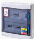
AC+DC distributor. Wall mounting, IP65. For operation of 3F FVE in combination with a switch (typically a GoodWe 4 to 10K-ET inverter). Manual transition from network and backup. It is necessary to control the load during a power failure to avoid overloading after switching the switch, because its function switches the whole house to inverter backup.
